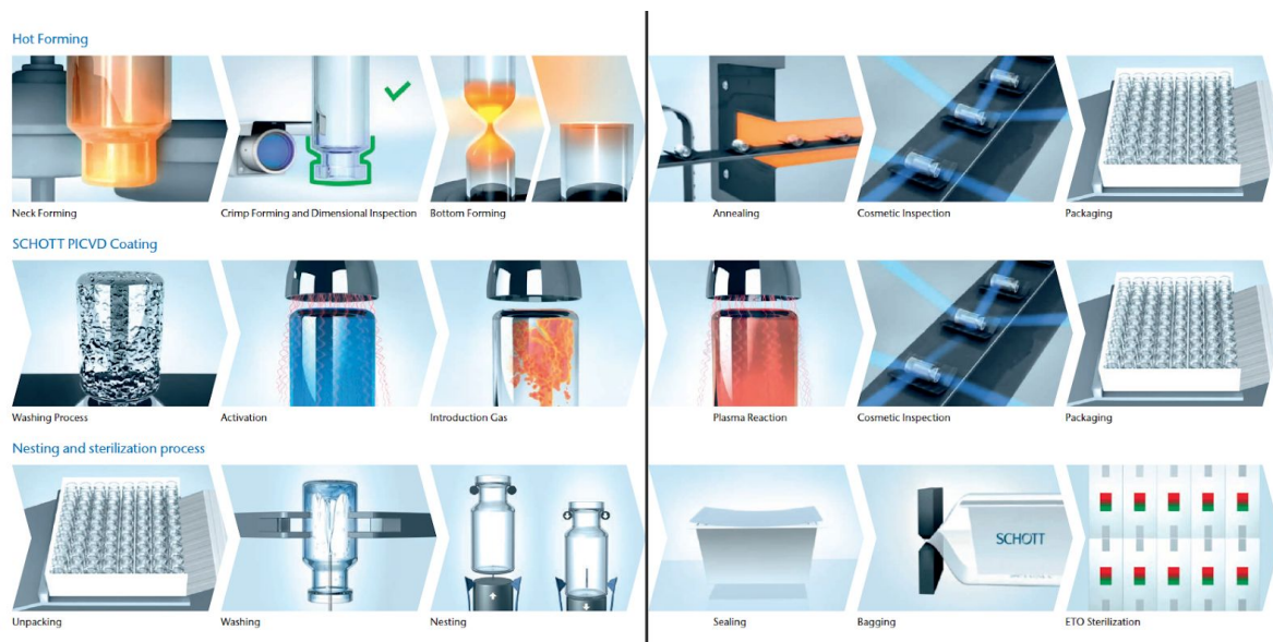
Figure 1: micro flow chart of the manufacturing process for glass vials. Source: SCHOTT Pharmaceutical Packaging 106
