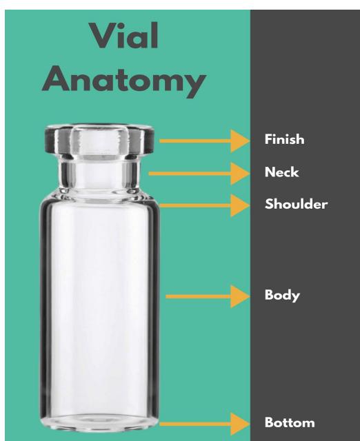
Figure 1: Vial anatomy. Data source: SCHOTT Pharmaceutical Packaging 82 . Image source: Gerresheimer 8
