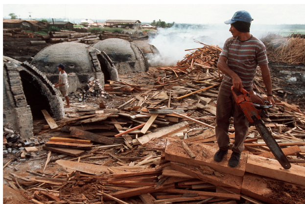
Scrap wood from a timber mill in Paragominas, Brazil, is burned to make cooking charcoal in beehive-shaped kilns. Photo (c) Joel Satore/joelsatore.com
