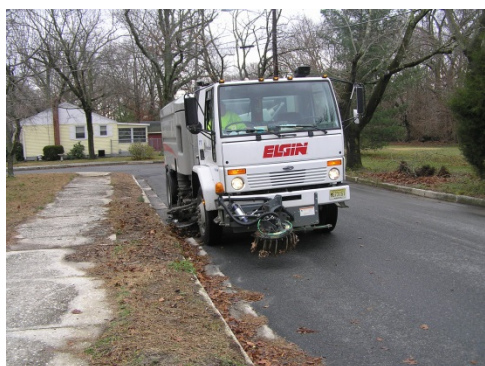
Figure 6. Mechanical street sweeping in Vineland, NJ (Source: City of Vineland, New Jersey).
