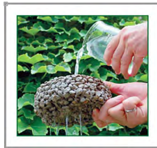
Figure 1: Image of water seepage through porous concrete. 53
