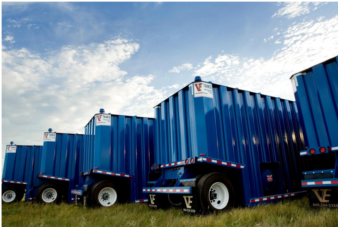
Figure 6. Closed-loop storage containers for hydraulic fracturing waste (VE Enterprises, Inc 2010).
