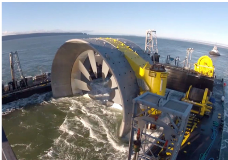
Figure 16: This photo shows an example of tidal stream energy generation in the Bay of Fundy, Canada. A tugboat (in the upper right-hand corner) is used to position the turbine towards the incoming tidal water. Image source: The Philadelphia Inquirer 77
