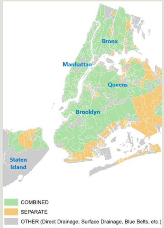
Figure 3.2.2 Sewer systems in NYC (Source: NYC DEP)
