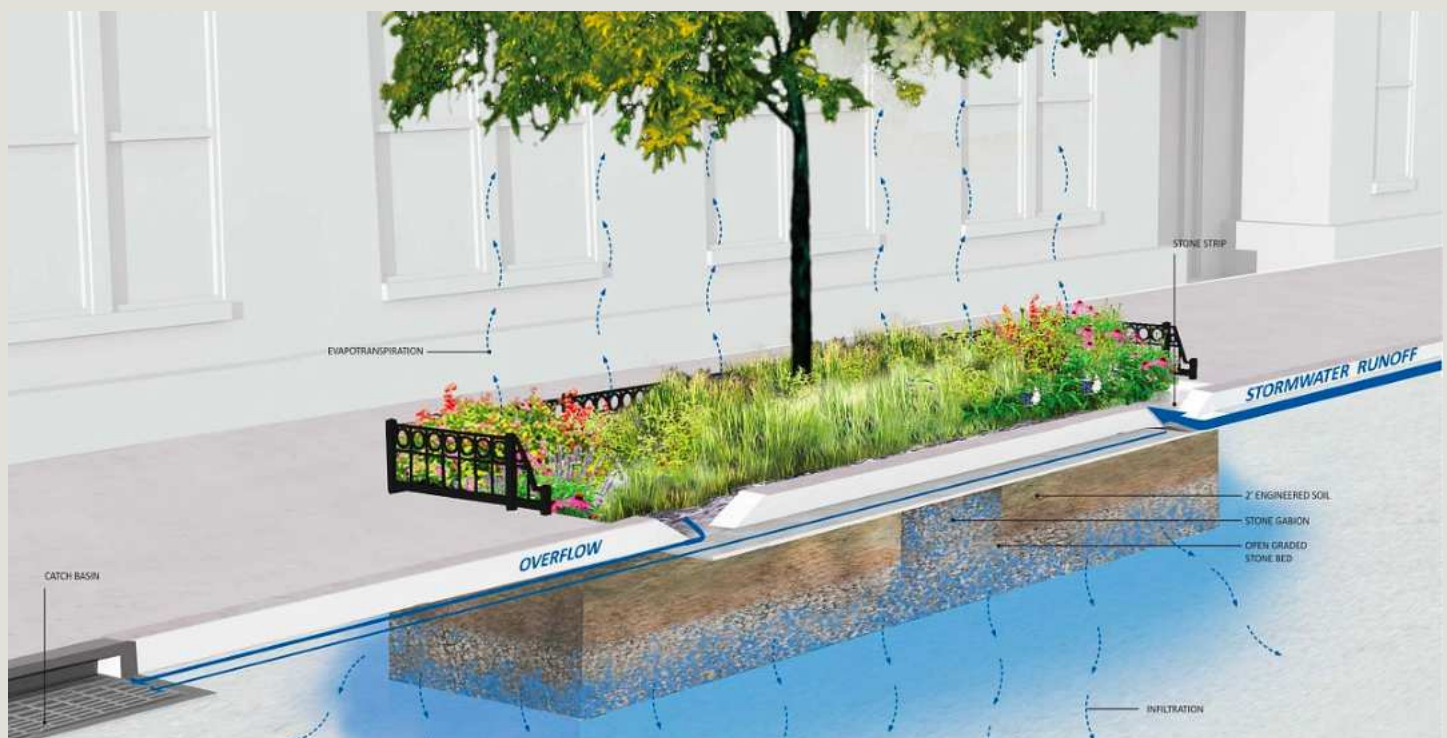
Figure 5.3.1.1 How a Bioswale Works
