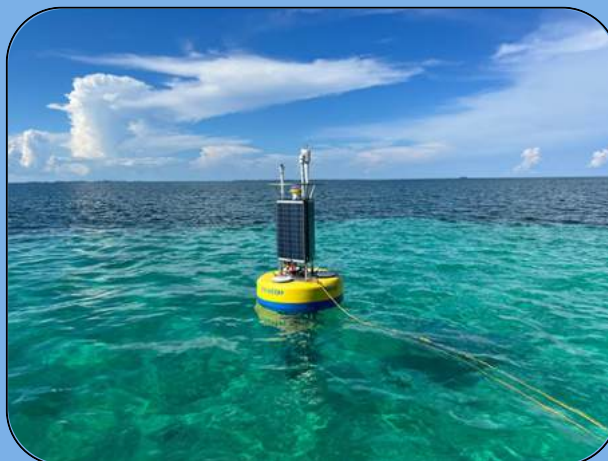
A solar-powered oceanographic buoy deployed in the Caribbean collects real-time climate and water quality data, supporting regional efforts to build climate resilience through sustainable monitoring technologies | Albert Jones / Caribbean Community Climate Change Centre (CCCCC) (Fondriest Environmental)
