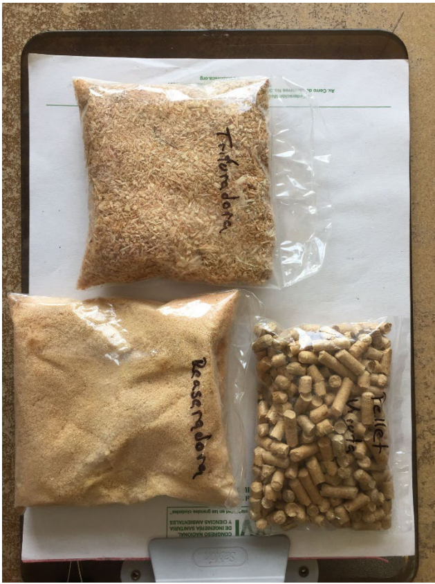
Figure 2: Pellets from Sawmill Production Waste in Durango Mexico. Photo by Myriam Amezcua
